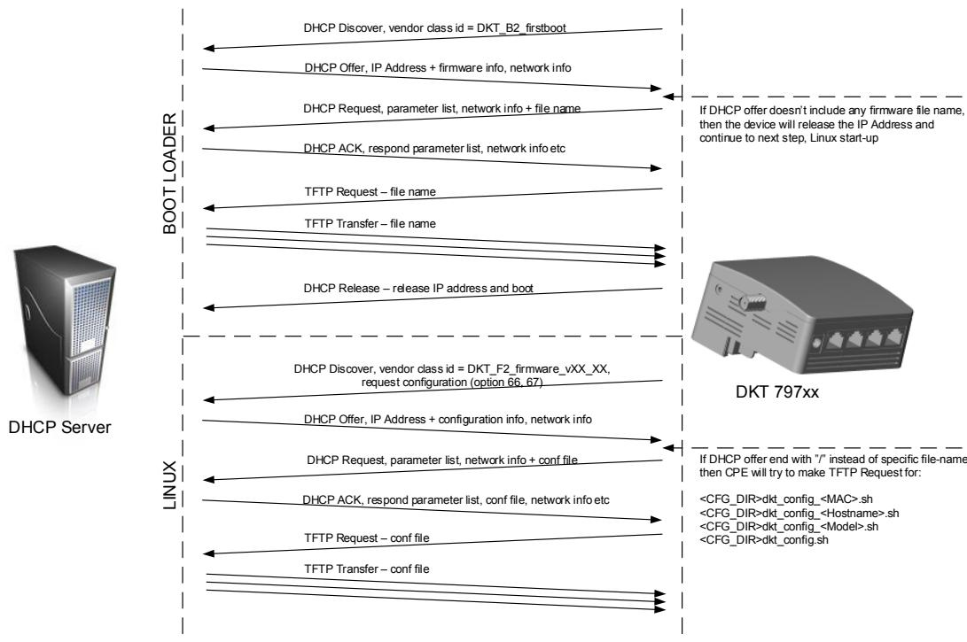
At device start-up configuration is provisioned automatically. Firmware is provisioned by request, either at first boot or when applicable
