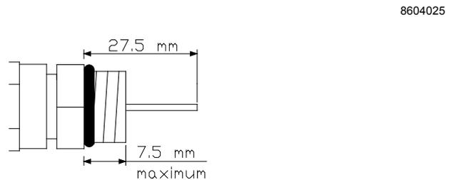
Figure 3. Centre conductor length
