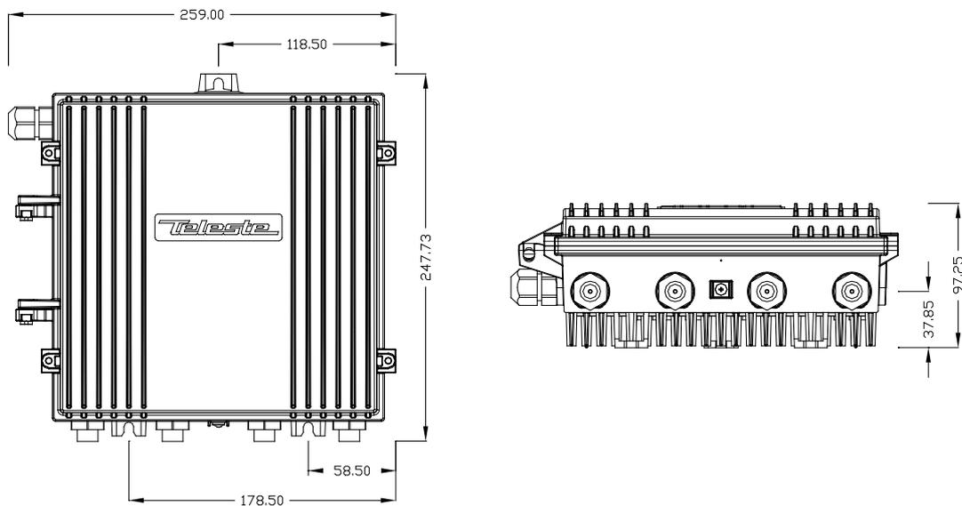
Figure 1. AC3200 housing dimensions – top side view
