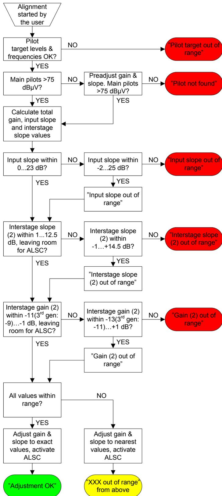
Figure 7. Simplified forward path automatic alignment flowchart
