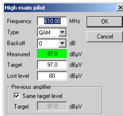
Figure 10. The pilot signal configuration dialog box
