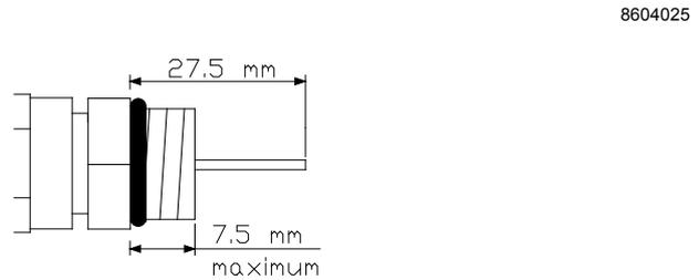
Figure 3. Centre conductor length
